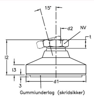
$\begin{array}{lll} d1 & = 40 \\ d2 & = M10 \\ l2 & = 25.5 \\ l3 & = 6.0 \\ NV & = 15.0 \\ Static load (N) = 10000 \\ t min & = 10.5 \end{array}$
